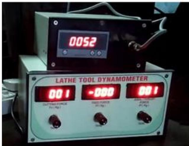
**Fig. 1: Lathe tool dynamometer**
