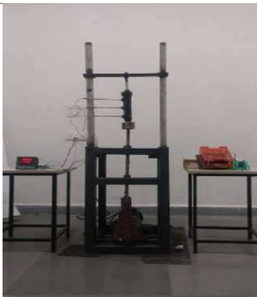
Figure 1: Experimental Set-up for Shock Absorber
