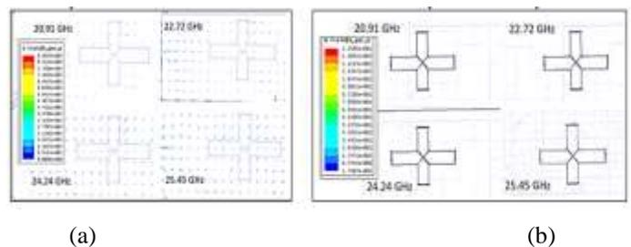
Figure7. (a) E-field distribution for four resonant frequency modes 20.91GHz, 22.72 GHz,24.24 GHz,25.45 GHz(b) H-field distribution for four resonant frequency modes 20.91GHz, 22.72 GHz,24.24 GHz,25.45 GHz
