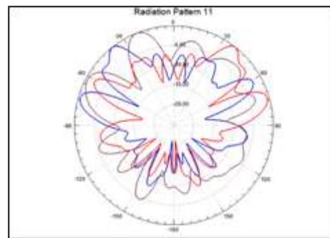
**Figure 4.** Radiation pattern of RDRA with cylindrical slot
