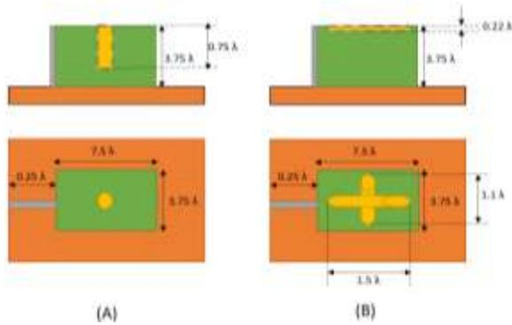
**Figure 1.** (A) RDRA with cylindrical slot filled with ethyl acetate
