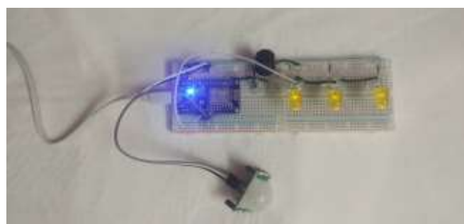
Fig 3.3 LDR is covered with black object its dark, but no movements detected so the Light is DIM
