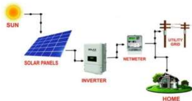
Fig 3.1 On-Grid solar system
