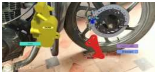
Fig. 12. User interaction – scaling up of a component (brake caliper)
