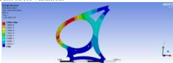
Fig. 10 Analysis of Motor mount (front)
