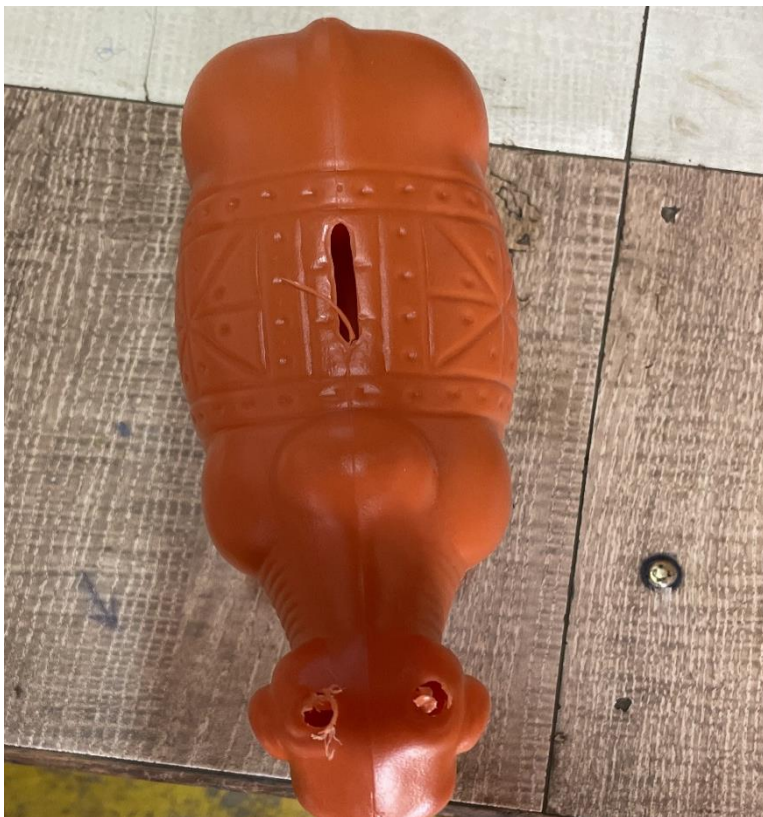
Figures in Clockwise Direction: - Image of 3D CAD Model of Cow Money Bank, Actual Assembled Model (With Horns) Cow Bank, Flash, Incomplete Shot and Dimensional Inaccuracy (Center), Burrs (Bottom Left), Flash, Sharp Parting Lines (Bottom Right)
