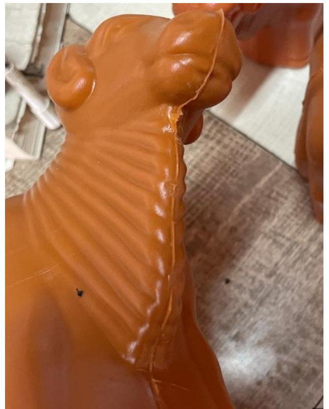
Figures in Clockwise Direction: - Image of 3D CAD Model of Cow Money Bank, Actual Assembled Model (With Horns) Cow Bank, Flash, Incomplete Shot and Dimensional Inaccuracy (Center), Burrs (Bottom Left), Flash, Sharp Parting Lines (Bottom Right)
