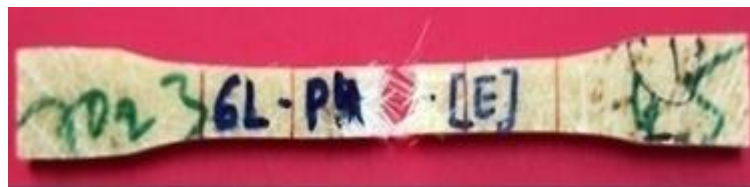
Figure 7: Fractured parts of the specimen tested in tension
