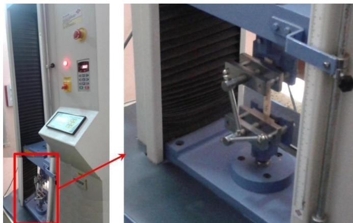
Figure 5: GFRP composite specimens under tension in UTM.
