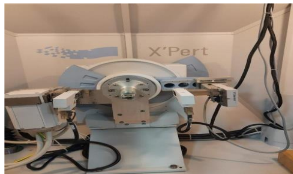
Figure 11: X' Pert Powder X-Ray Diffraction Machine
