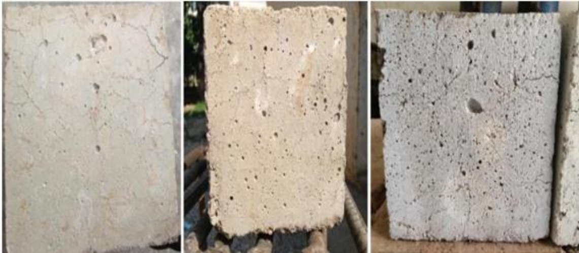
Fig. 9: Specimens exposed between 600°C to 800°C
