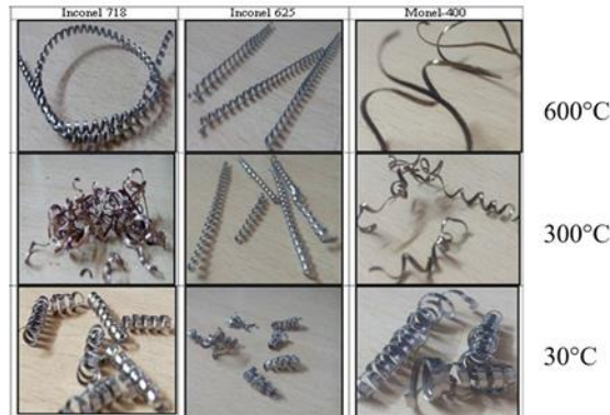
Figure 3. Chip formation in different three materials [5]
