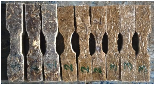
Fig 2.1 specimen as per ASTM D638
