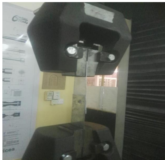
Figure 1 Tensile test of PVC composite film
