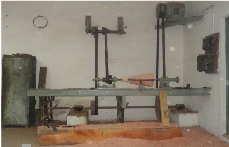
Figure 2.1 Set -up used to make the pattern of Socket
