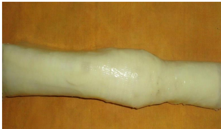
Figure 2.6: Shin made of Glass-Epoxy composite
