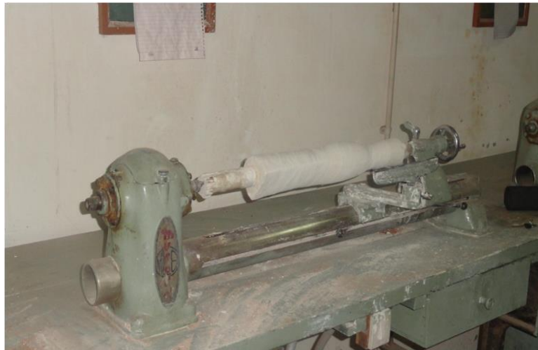
Figure 2.2 Set-up used to make the pattern of shin
