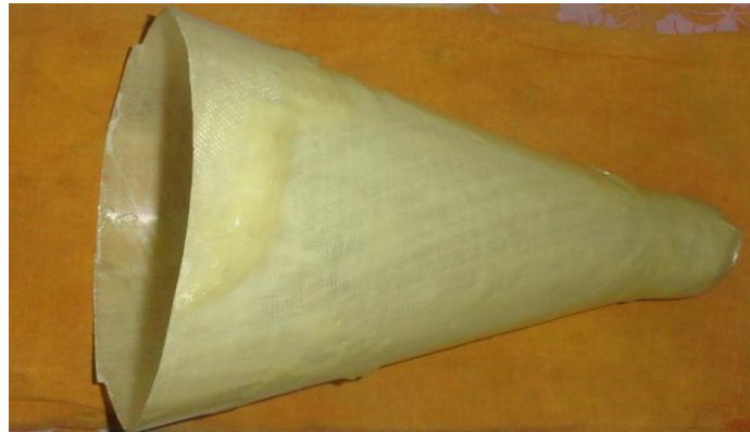
Figure 2.5: Socket made of Glass-Epoxy composite
