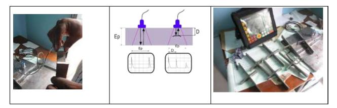
Fig 6. Ultrasonic Testing Procedure
