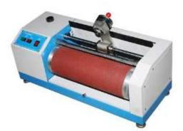
Fig 7.Wear Testing Equipment
