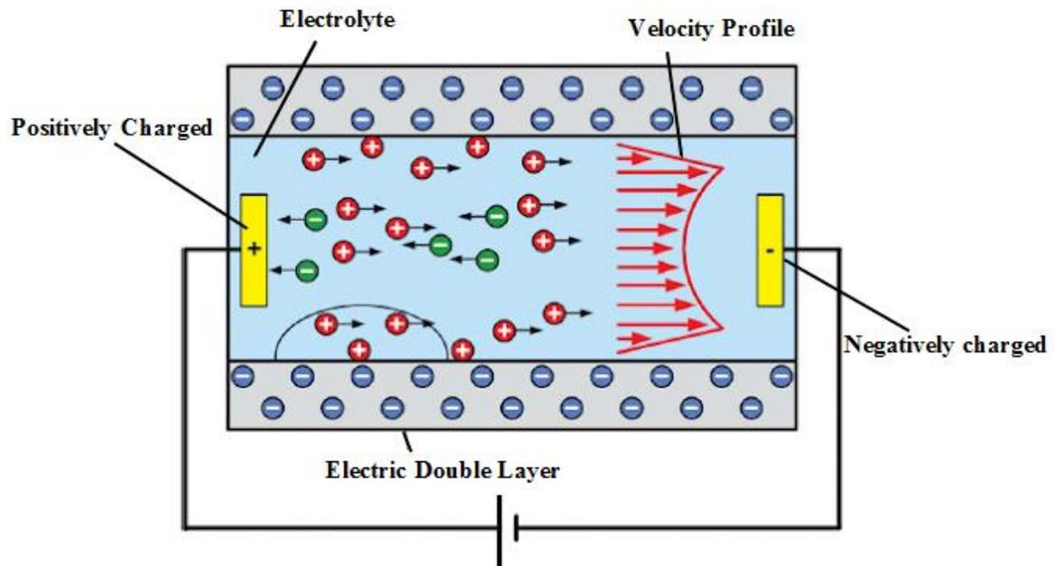
**Figure 2:** Schematic diagram of electro osmotic fluid flow in micro channel
