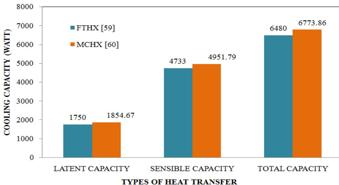
**Figure 3:** Comparison of the cooling capacity of FTHX and MCHX
