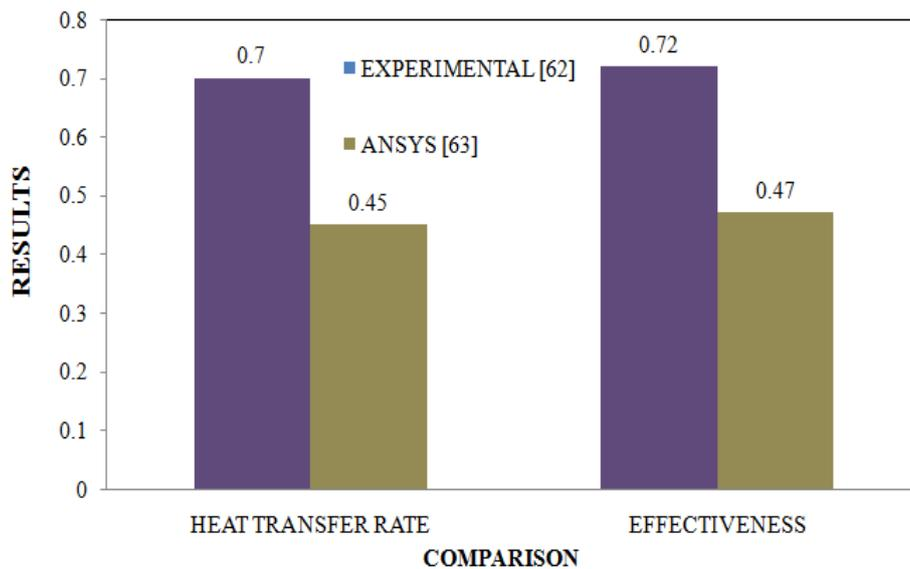
**Figure 5:** Comparison of the heat transfer rate (kW) and effectiveness using the results (Experimental and ANSYS)
