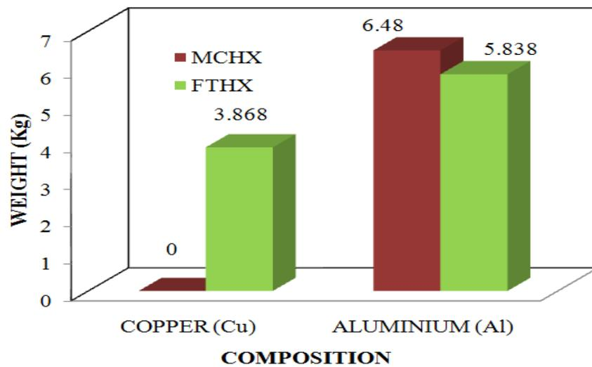
**Figure 4:** Composition of Cu and Al in the FTHX and MCHX
