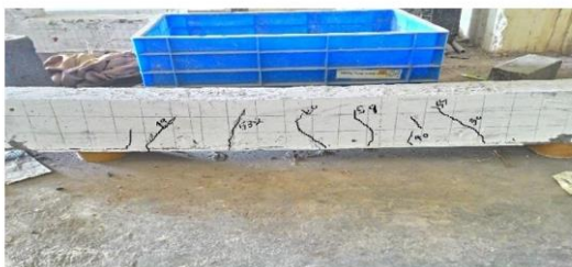
Fig. 8(b): Crack pattern for GGBS and BA
