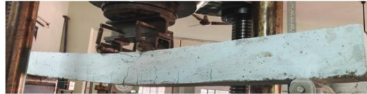
Fig.17 Four point loaded beam sample for flexure test (FDB)
