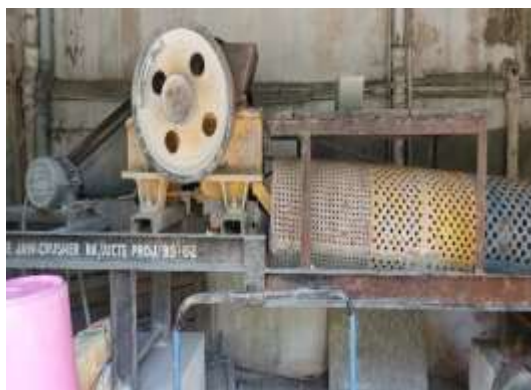
Figure 1: Recycled Aggregates Crusher and Processing Unit (Attached sieving unit)
