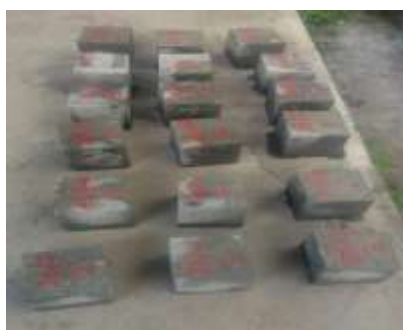
Figure 2: Standard Cube specimens kept for air drying before testing
