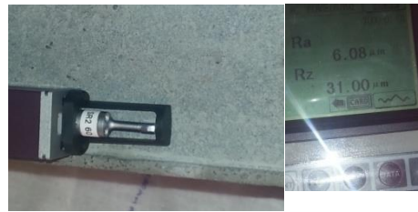
Figure12. Roughness measurement on new untreated concrete
