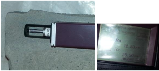
Figure11. Roughness measurement on new treated concrete
