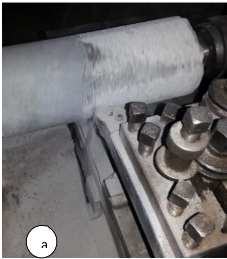
Figure7. Carriage machining of the treated ingot (a), grooving of the treated ingot (b)
