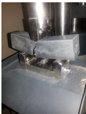
Figure 3 HPFC and HPC three-point bending tests
