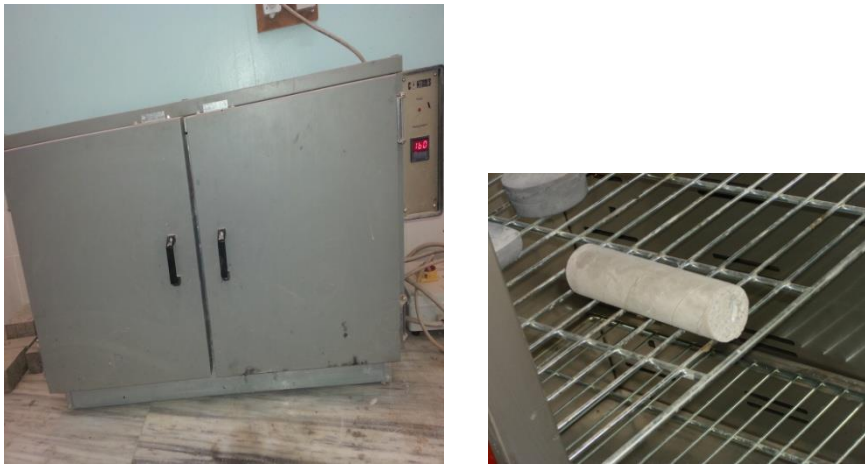
Figure4. HPFC ingot Treated at 160 ° C for three days.
