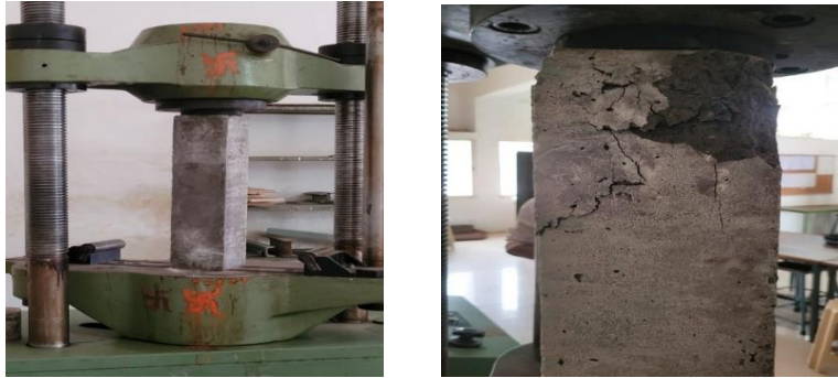
Figure 3: RCC Column Placed Under & UTM Crack in RCC column at the ultimate load
