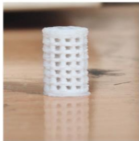
Fig. 4. 3D printed PLA specimen (Experiment no 27)
