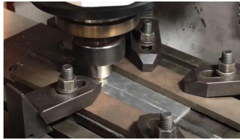
Fig. 1 Shows Schematic representation of FSW process
