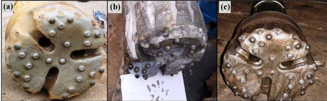
Fig. 8. The three possible failure modes of the hammer bits are (a) tooth loss, (b) tooth fracture, and (c) tooth wear, according to Fan et al. (2011).
