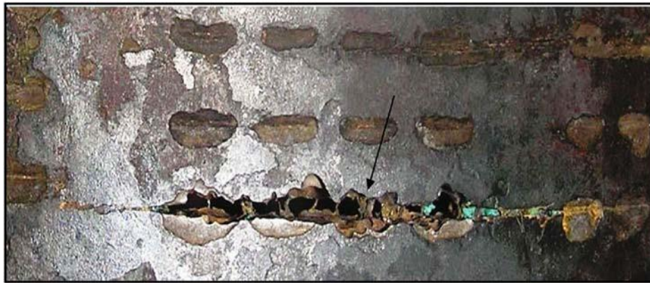
Figure 5 (Moradi and Ranjbar, 2009) shows how die marks affect the failure of drill pipes.
