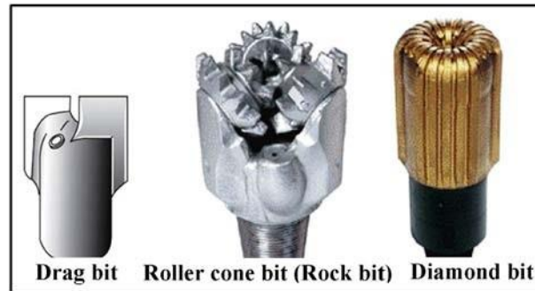
Fig. 9. Sorted categories for drilling bits (Wamsley Jr. & Ford, 2006).
